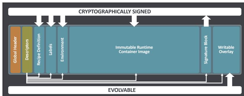
Figure 2: Singularity Image Format file structure and usage
