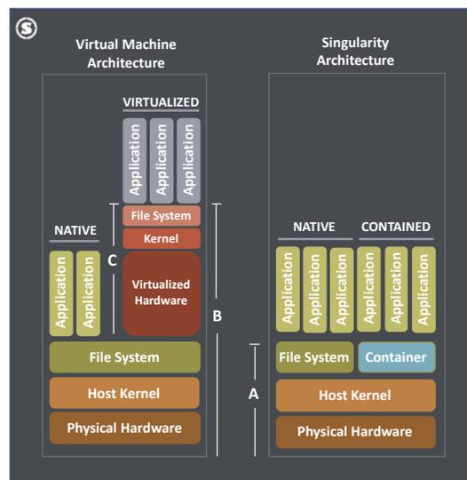
Figure 3: Positioning of Singularity in a Linux system
